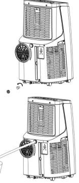
**Note:** This model has a self-evaporative function, which reduces the need to empty the water tank. If the unit is vented correctly most of the water is reused to cool the condenser coils and any excess is evaporated. Please do not use continuous drainage if you intend to use the self-evaporating facility.
