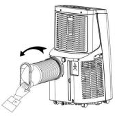
Extend one head of the hose and screw it into the unit anti-clockwise. The hose can be removed by screwing the hose clockwise. Note: to screw it into place should take no less than three rotations.
