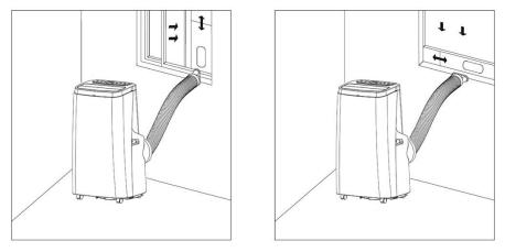
**Note:** The window kit is only designed to be installed with sliding or sash windows or doors. The window kit is not designed or to be used with any other style of windows. However, the fish tail adaptor can be used with most windows / doors. When using the cooling mode ensure that the opening left is as small as possible. The best form of installation is through a wall duct. By properly venting, you expel hot air from your room while efficiently cooling it.
